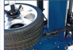
The bead-breaking is performed by means of an EASY ROLLER:
