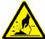
**When clamping the rim, do not place hand or other parts of the body in between the clamp & the rim.**
