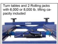
Chain driven for strength and durability. Pneumatically operated safety locks engage and lock/unlock every few inches. 3 front turn table position and built in /flush mount slip plates accommodate short as well as long wheel base vehicles.
