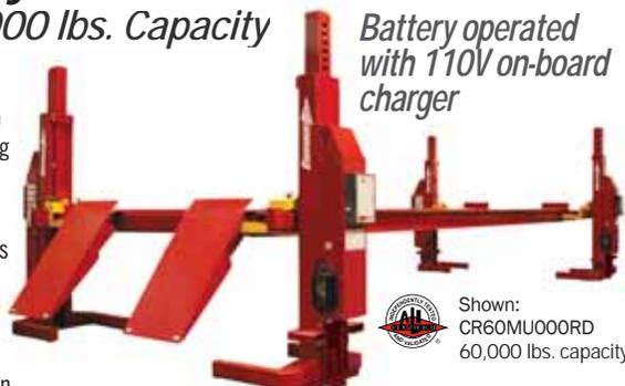
Battery operated with 110V on-board charger
