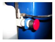
5.Connect shop air to palm valve. We recommend using leftover hose and NPT fitting (not included).
