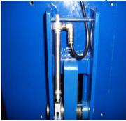
2.Run air hose up and over top of column, running through top side of overhead beam and down to main side lock assembly.
