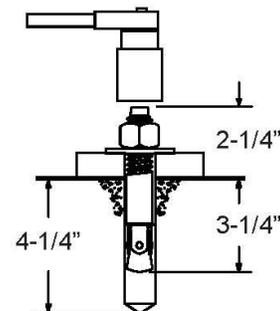
Tighten nut with Torque wrench to 130 ft.-lbs.
