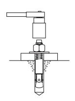
Tighten nut with Torque wrench to 40 ft.-lbs.
