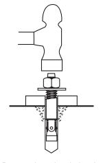
Run nut down just below impact section of bolt. Drive anchor into hole until nut and washer contact base.
